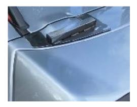
Start by cleaning the area where the bracket will be installed. With rear hatch door shut, place and stick top bracket parallel with outer edge of stock roof rack. Make sure to align back edge of bracket with spoiler to fit as shown in **photo 1**.
