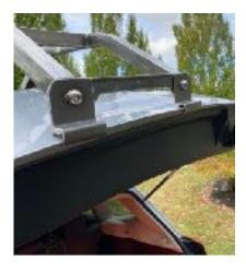
With rear door open, align bottom of the ladder parallel to the bottom of rear hatch door. Attach bottom bracket, with provided screws, to base of ladder, over the lip of the bottom door hatch, as shown in **photo 3.**
