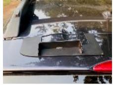
Start by cleaning the area where the bracket will be installed. With rear hatch door shut, place and stick top bracket one inch to the right of the inside edge of roof rails as shown in **photo 1**.
