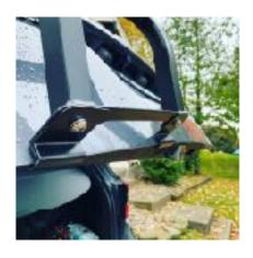
With rear door open, align bottom of the ladder parallel to the bottom of rear door. Attach bottom bracket with provided screws to base of ladder (over the lip of the bottom door hatch), as shown in **photo 3.**
