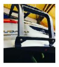
With rear door just slightly open, align bottom of ladder to the bottom of rear door. Then, attach bottom bracket, with provided screws, to base of ladder and over the lip of the door as shown in **photo 3**.
